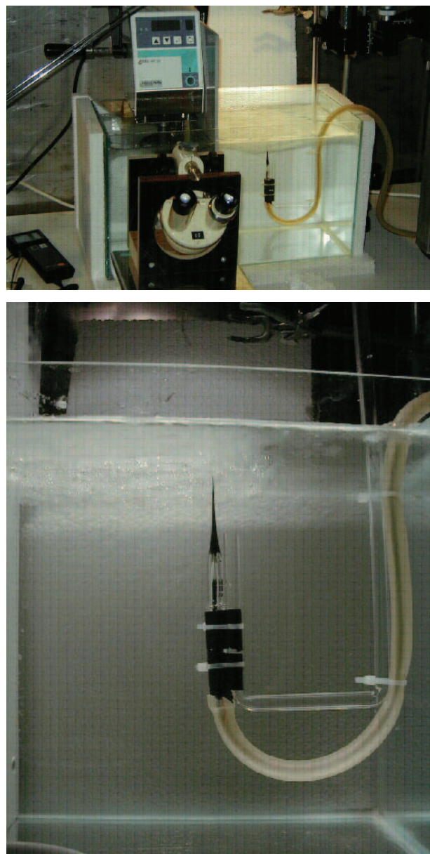
Fig. 1. Experimental set-up used to study the O 2 dynamics at the ice-water interface. The temperature of the water and air could be controlled independently ( \pm 0.2^\circ\text{C} ). Lower panel represents a close up of the upper panel
