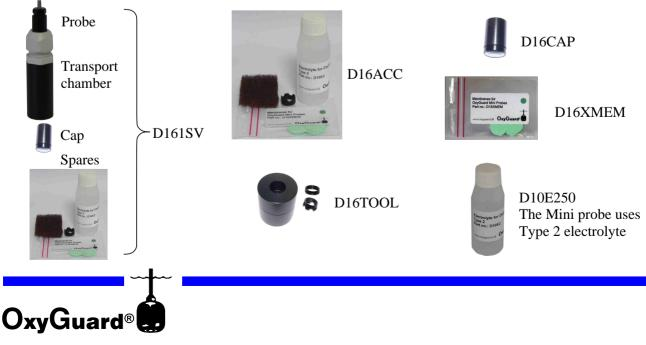
**<u>Probe Renovation</u>** should only be performed if the membrane is damaged, or if it is not possible to calibrate to the correct value after a long period of use. It should NOT be performed on a regular basis.
